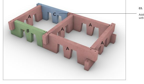
Add Parts A and C. Connect with corner rods.
